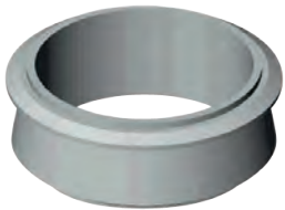
180.X.000040 - EM sleeve For mounting with a minimal footprint in supports or supporting cross bars. Hole diameter: 87 mm - 90 mm. Material: EPDM
